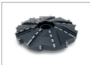
Diamond mushroom shaped peripheral milling tool - with flutes, spring loaded + flushing holes - Field of application: Removal of intruding laterals and deposits
